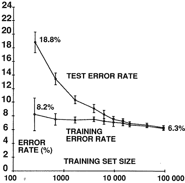
Figure 1: Training and test error rate for a boosting network using three 100-10-10 networks.
